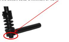
Step 4. Adjust the position of the dynamic coil spring with a footplate attached to the support tube in order to accommodate the knee-to-heel distance required for the client. Tighten the collar fasteners to secure in place.
